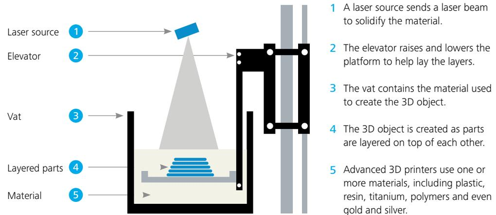
Due to the inimitable manufacturing processes of 3D printing, people now have the ability to innovate products from the inside out. The process cannot be mimicked using traditional manufacturing methods, since 3D printing is an additive process. This means that individuals and businesses alike can create internal skeletal structures and unique shapes within an object.
