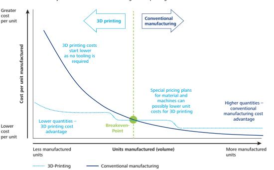
The break-even point is where the two cost curves intersect. At present, conventional manufacturing offers cost advantages when volumes and production runs are high, although this is likely to change. 3D printing is, by contrast, **attractive even for small volumes**. Special pricing plans for materials and printers may well bring unit costs down in the long term.
