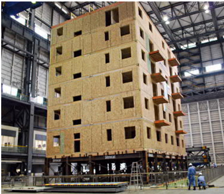
Figure 4 – Six story timber building on shake table (credit: Colorado State University)
