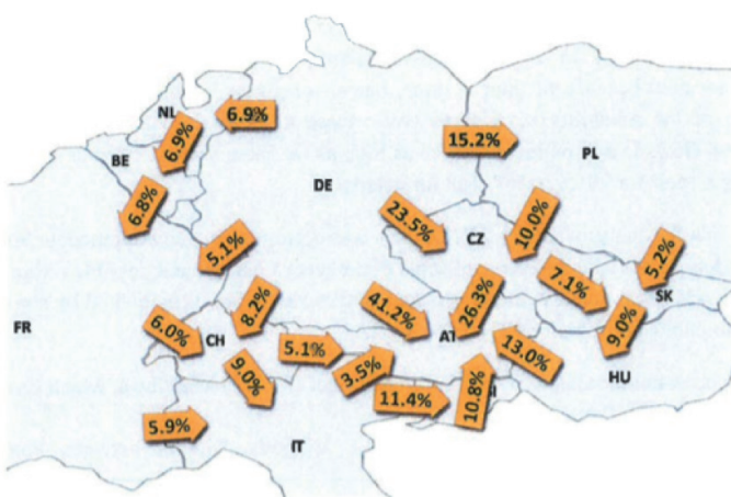
Figure 2 : Distribution of the physical flows of electricity for a commercial trade from Germany to Austria (source: ACER 3 )
