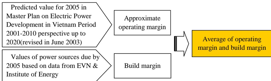
Figure-4 Calculation method of baseline (Emission coefficient)
