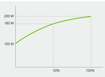
Figure 2: The non-linearity of utilisation and power.<sup>12</sup>
